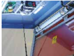
Isolated electrical components assembly from contaminated zones, easy to reach for servicing
