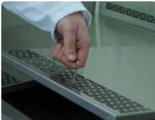
Removable monoblock or sterilization available partitted, high strength, non-vibrating stainless steel work plate
