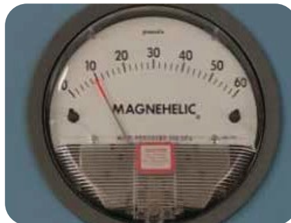
Magnehelic work chamber negative pressure gauge
