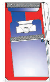
Plenum cast design creates negative pressure around contaminated work area and ensures zero leakage
